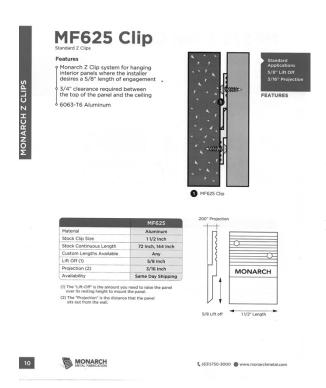
Cosmopolitan panels may be installed using Z Clips and Z Bars. Although the ultimate choice of the installation system is subject to the installer's discretion, many customers have successfully used the Monarch MF625 Z Clips for installation. This Z Clip provides a 3/16" projection with a 5/8" lift off.
